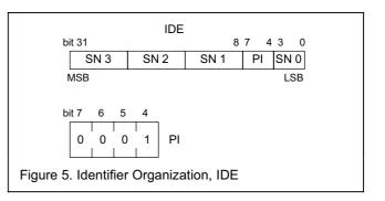
The Identifier, IDE, is incorporated in the process of device authentication and used by the on-chip Calculation Unit as well as by the interrogating system.
