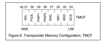
The memory access rights applied by TMCF affect the behavior of READ\_PAGE and WRITE\_PAGE commands only. Device operation, e.g. with respect to the authentication process, is not affected at all.
