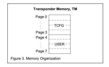
The TM segment can be accessed only, after successful device authorization. Depending on the device configuration, device authorization is performed either in Password mode or in Cipher mode. Subsequent memory access is provided only in accordance with the memory protection settings applied.
